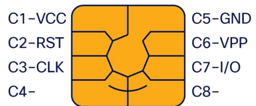
Figure 2: Smartcard pinout diagram
